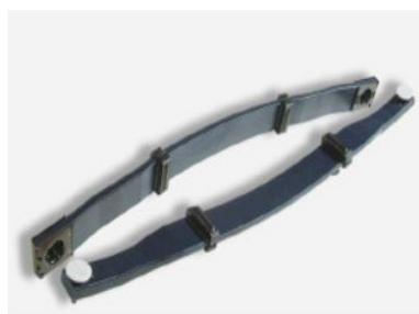
Carbon fiber composite leaf springs
